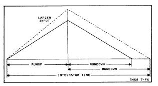
Figure 7-F-6. Dual Slope Conversion
