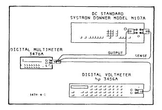
Figure 4-2. DC Volts Accuracy Test and Calibration
