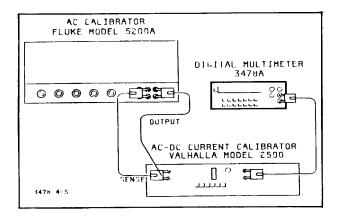
Figure 4-5. AC Current Accuracy Test and Calibration
