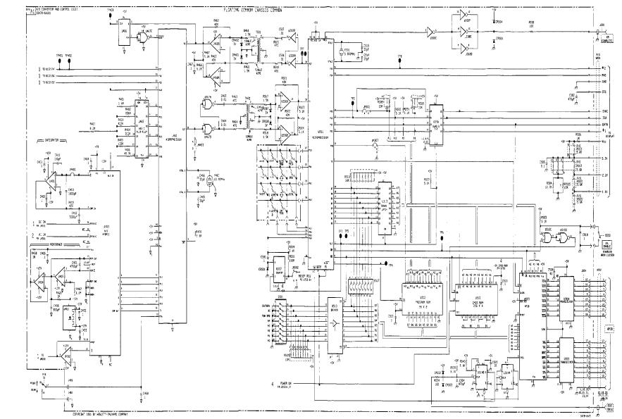
3 Figure 7-G-5. A/D Converter and Control Logic **7-G-9**
