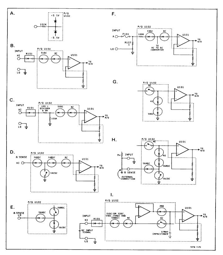
Figure 7-F-2. Simplified Schematic Of The Input Switching Circuitry
