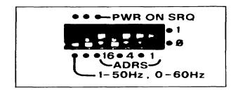
Figure 2-1. Line Frequency Switch
