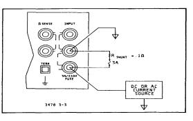
Figure 3-3. Typical Current Measurement Connection 3-15. Input Terminals Cleaning
