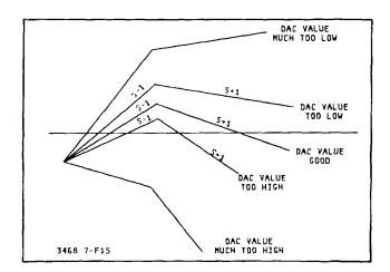
Figure 7-F-15. Determining the DAC Setting
