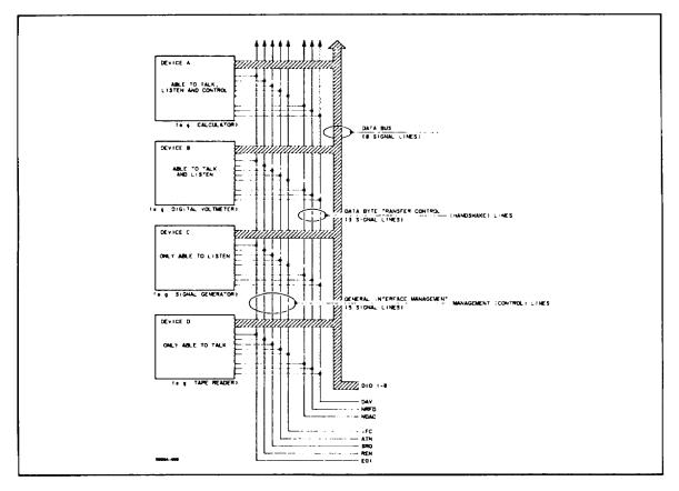
Figure A-1. Interface Connection and Bus Structure
