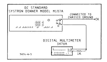
Figure 4-3. DC Common Mode Rejection Test
