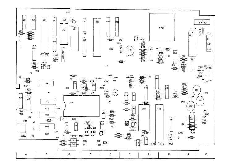
Component Locator for Input Circuitry and Ohms Current Source
