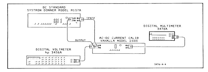
Figure 4-4. DC Current Accuracy Test and Calibration
