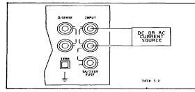
Figure 3-2. Typical Input Measurement Connection
