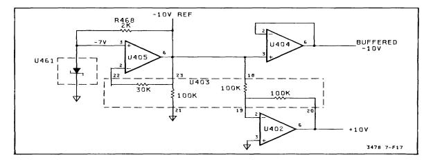
Figure 7-F-17. 3478A Simplified Reference Circuitry
