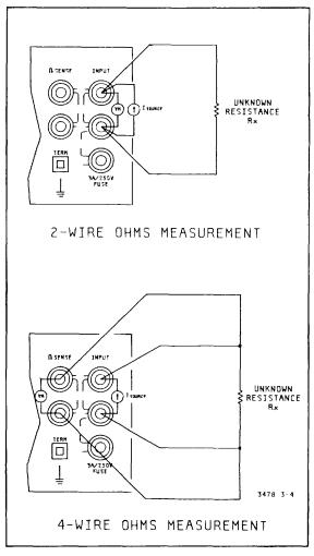
Figure 3-4. Ohms Connections
