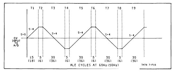
Figure 7-F-10. Runup Slopes for Zero Inputs (41/2 Digit Model)
