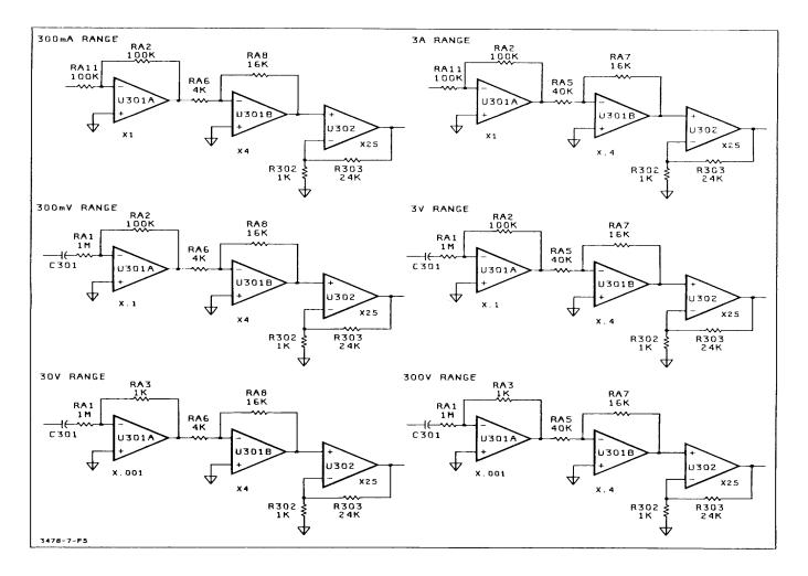
Figure 7-F-5. AC Gain Configurations
