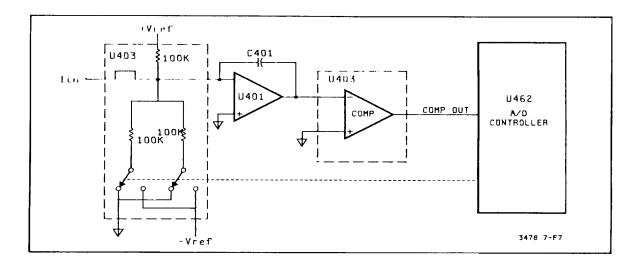
Figure 7-F-7. Simplified A/D Converter
