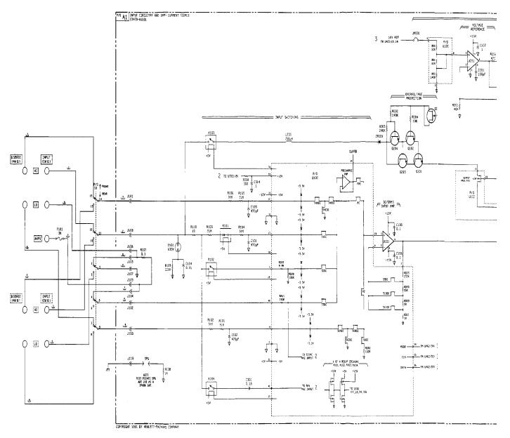
Figure 7-G-3. Input Circuitry and Ohms Current Source 7-G-5
