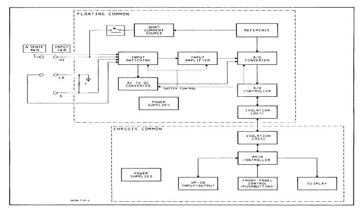
Figure 7-F-1. 3478A Simplified Block Diagram
