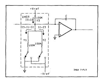
Figure 7-F-13. Slope S+0 and S-0 Generation
